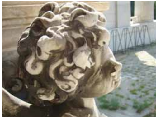
Fig. 5 Detail of marble sulfation. Photo by Caranza.
